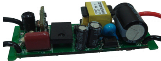
Figure 4: CXA1512 retail track light driver
